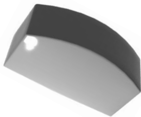
A chamfered box with a 3x3x3 FFD applied to round off the surface.
