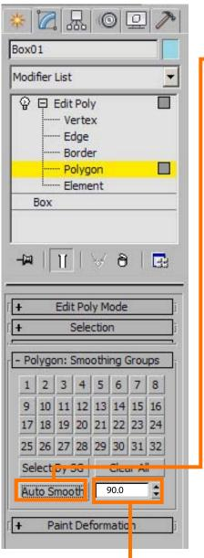
2. The angle setting determines if the polygons will smooth. for example, 90° is a good setting.
