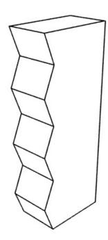
1. The first step to smoothing a grip like the one to the left is to "chamfer" the corners.
