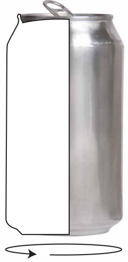
Lathing Spins the Spline Around an Axis and into a 3D object
