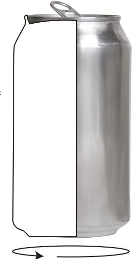
Lathing Spins the Spline Around an Axis and into a 3D object
